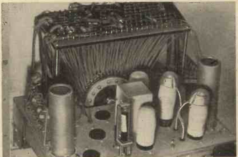
Top view of chassis showing connections from uniselector switch to impedance standards.
